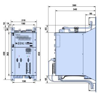
Fastening with 4 M6 hex-socket head screws.
